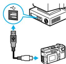
4. Connect the camera to the computer using the USB cable.
